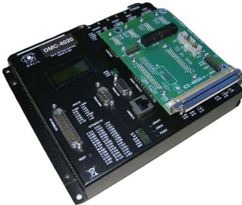
Figure 1: ICS-48100 mounted on top of DMC-40x0
