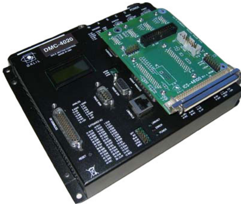
Figure 1: ICS-48100 mounted on top of DMC-40x0
