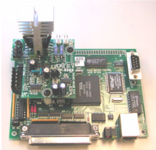
AMP-14120-1A mounted to the DMC-1425
