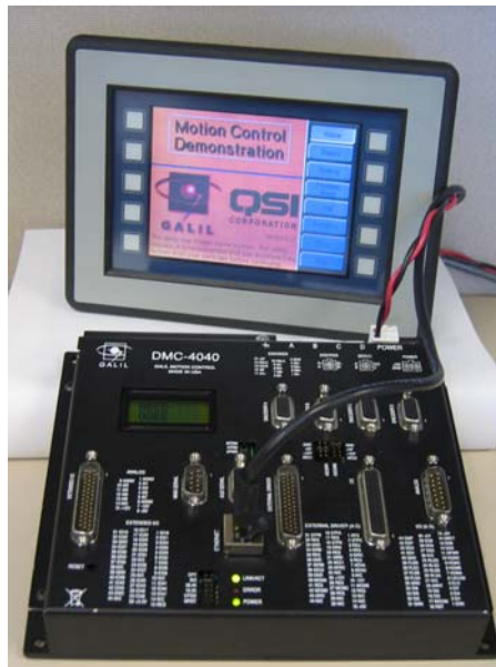
Figure 1: QSI GS124 Touch Screen HMI, connected to a Galil DMC-4040 Accelerera Series controller.
