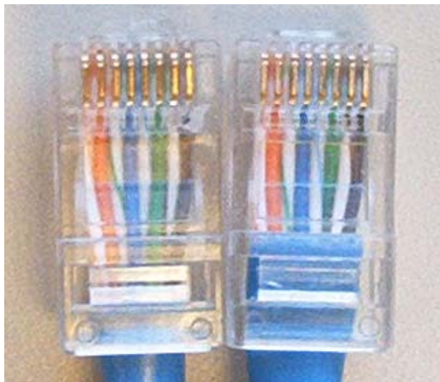
Figure 3. The ends of a straight-thru Ethernet cable. Side by side, the color code is the same.
