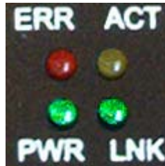
Figure 5. Controller indicator lights for DMC-14x5, 34x5, or 1416 (LED positions for 21x2, 21x3, and 31x3 are the same)
