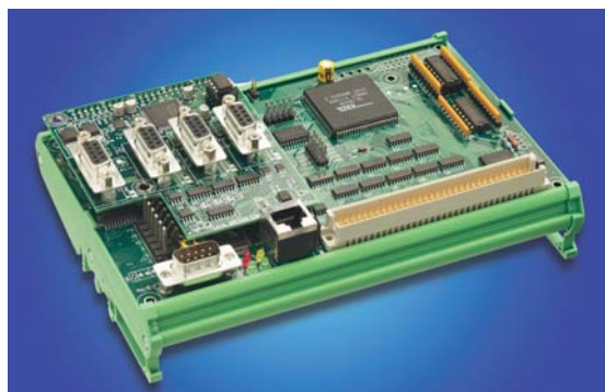
DB-28104 Sinusoidal Interpolation board attached to a DMC-2143 Ethernet Motion Controller.
