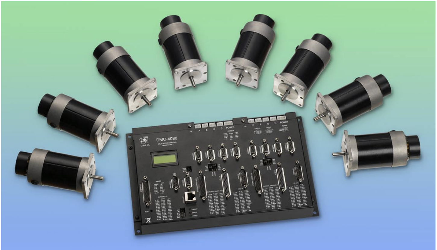
DMC-4080 8-axis controller and drive unit operates eight motors.
